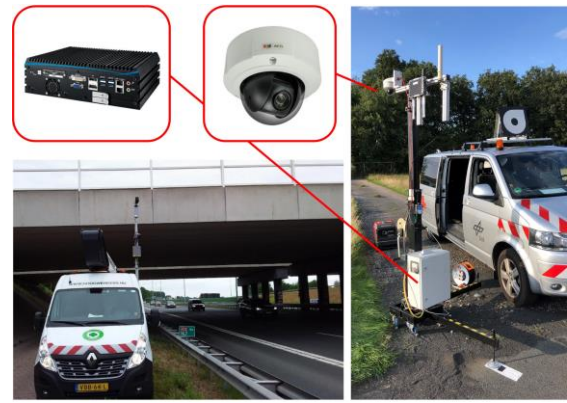
Fig. 3. Used mobile poles, equipped with cameras, RSUs and workstations on the test track (right) and on the highway (left)
