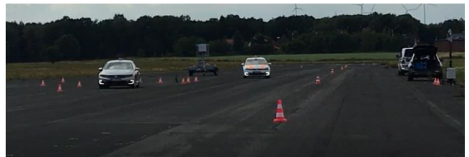
Fig. 7. Cooperative lane change of the highway CAV (middle) driving on the virtual highway in UC 2.1., when the merging CAV (left) tries to change lane. Infrastructure gives an early speed advice to the on-ramp vehicle. Then, both vehicles coordinate the lane changes by using the MCM-V2V cooperation.
