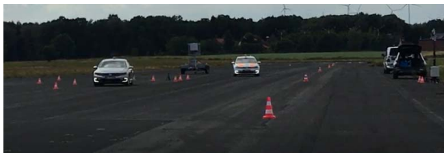
Fig. 7. Cooperative lane change of the FASCarE (middle) driving on the virtual highway in use case 2.3., when the ViewCar2 tries to merge. Infrastructure gives an early speed advice to the on-ramp vehicle. Then, both vehicles coordinate the lane changes by using the V2V-MCM-cooperation.
