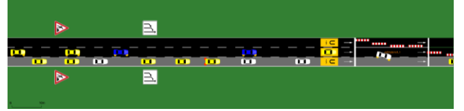
Figure 3. Detail view of the merging area in SUMO for scenario 1. The grey lane is usually reserved for public transport but opened temporarily to provide a possibility to pass the construction works stretching over the two main lanes. Vehicle colours indicate the vehicle type (yellow for legacy vehicles, blue for CAVs, and white for CVs).
