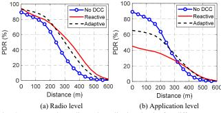
Fig. 3. PDR at the radio and application levels for different DCC configurations, when all packets have the same priority (DP2). Traffic density: 180 veh/km.
