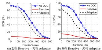
Fig. 5. PDR (Packet Delivery Ratio) at the application level for scenarios with a mix of vehicles using Reactive and Adaptive, when all packets are configured with the same priority (DP2). Traffic density: 120 veh/km.
