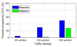
Fig. 2. Packets dropped by DCC for different traffic densities and DCC configurations, when all packets are configured with the same priority.
